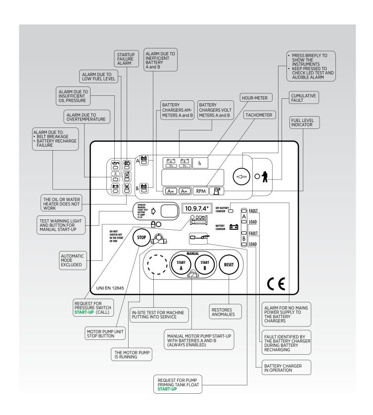
Figure 3. Control Panel Buttons and Indicators
